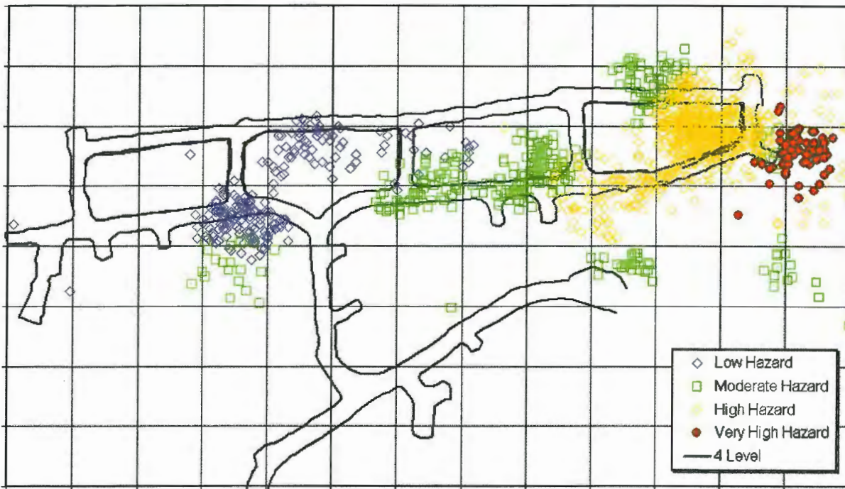
Figure 46: Seismic events displayed on a mine plan indicating areas where the rock mass is failing
