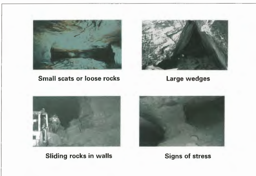
Figure 35: Example of an excavation assessment sheet designed to assist jumbo operators and ground support crews in informal daily rockfall risk assessment
