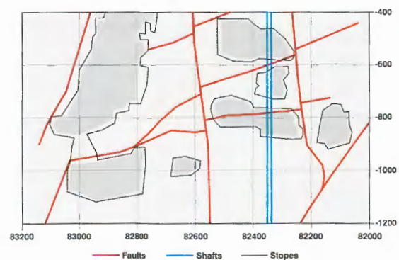
Figure 2: Generic section of a mine showing a network of major geological structures
