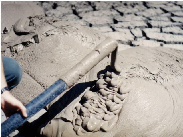
FIGURE 1.3 Examples of ultra-high density (paste) thickened tailings
