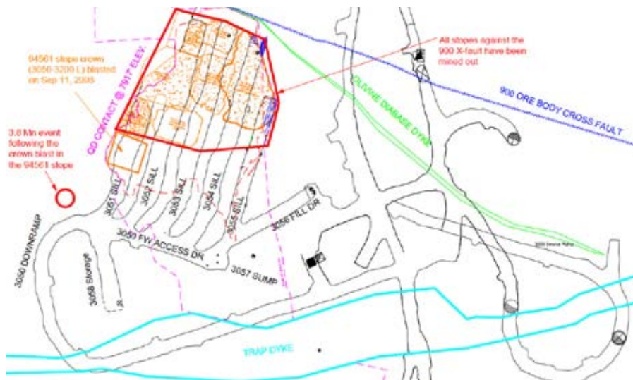
Figure 3 Layout showing the location of trap dyke and 900 X-fault in relation to mining between 3050 and 3200 L
