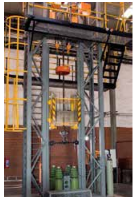
Figure 2 The DIT, as installed
