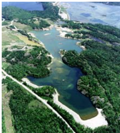
Tailings area after remediation by flooding
