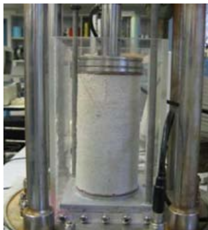
Figure 2 UCS test with specimen submerged in water bath
