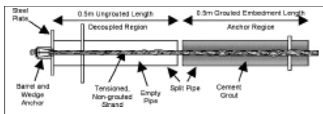
Figure 1 Schematic representation of split pipe testing system
