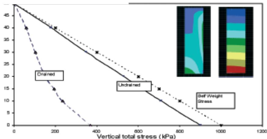
Figure 1 Predicted variation of vertical total stress along the centreline of a slope filled with uncemented tailings. Results are shown for the fully drained and the undrained condition
