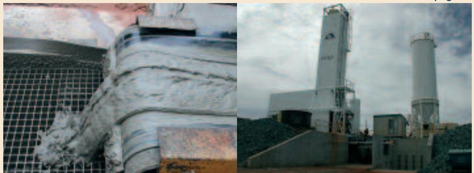
Industry has witnessed an increased use of full-plant tailings as backfill. In some cases, cement and other binders are added to produce paste fill. Photos courtesy of St Ives Gold
