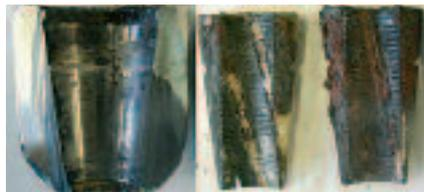
Figure 4 Internal condition of barrel and three-part wedge anchor that did not fail after 10 months in corrosion chamber
