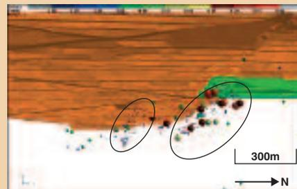
Figure 5 Planned seismic array at Xstrata Zinc's Black Star open cut. The planned pit geometry in relation to the known subsurface cavities is as shown
