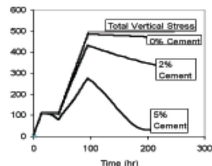
Figure 5 Impact of changes to cement addition
