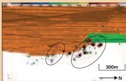
Figure 2 Total events recorded over the monitoring period, scaled to Moment Magnitude and with significant clusters highlighted
