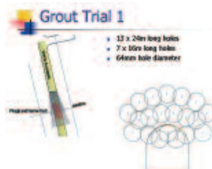
*Grout trial one grout holes*
