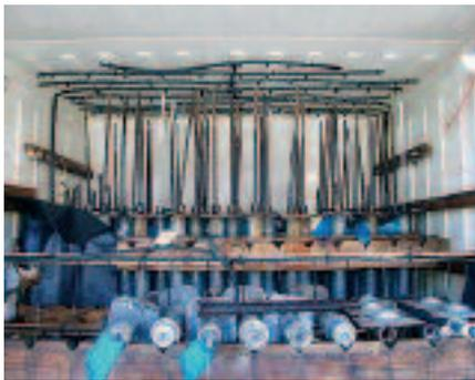
Figure 2 Corrosion chamber displaying barrel and wedge testing at rear
