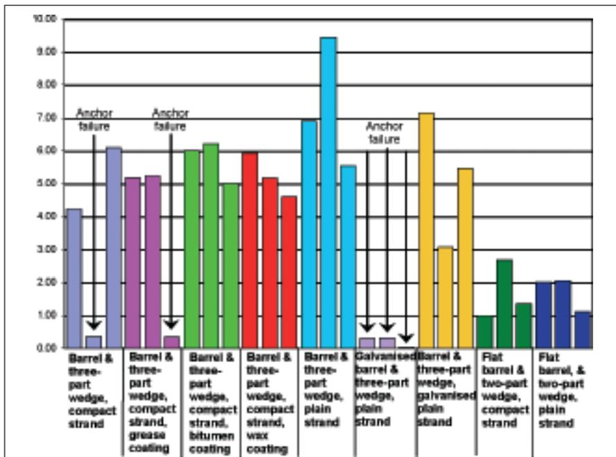
Figure 5 Total wedge movement of anchors after 10 months in the corrosion chamber
