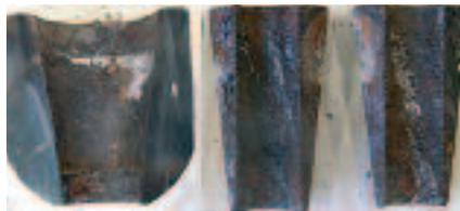
Figure 3 Internal condition of failed barrel and three-part wedge anchor. Note the corrosion on the barrel surface and the shearing of the wedge teeth
